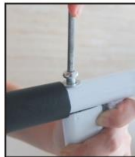
3. Fix handle with long screw
